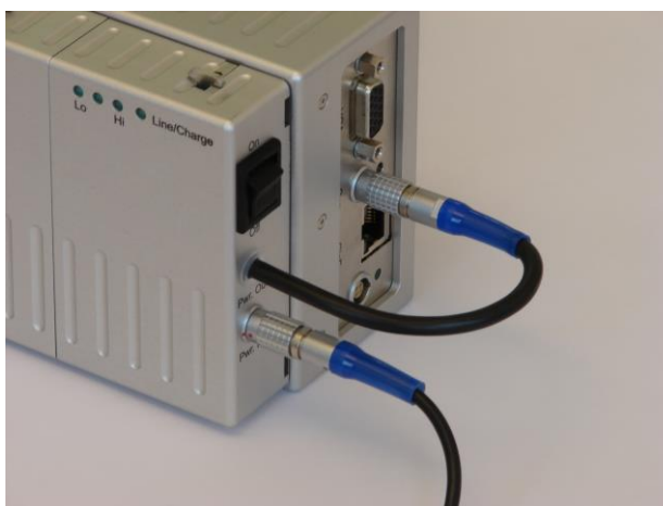
Schritt 6: Switch should be in positioned in „off“ state, connect camera and AccuPack
