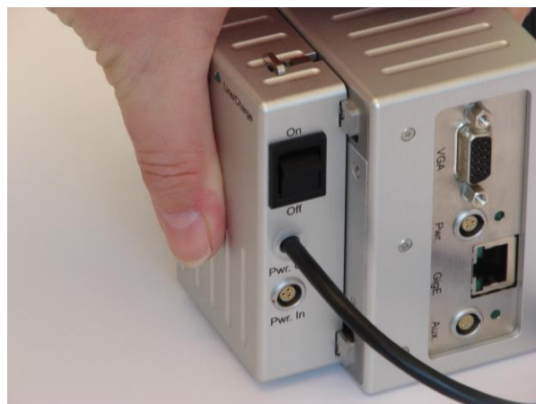
Step 2: Push Charger to backside
