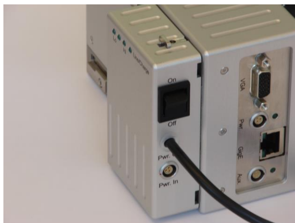
Step 3: Shift Charger into locking position
