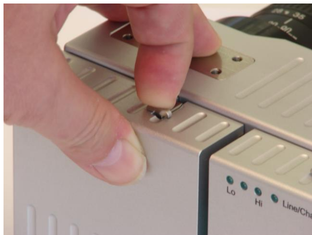
Step 9: ... and shift Accumulator to the left
