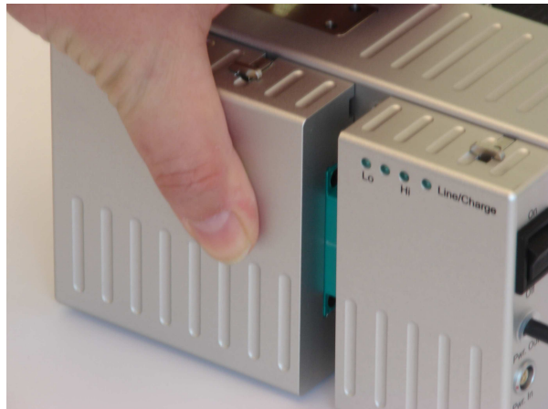
Step 4: Attach Lilon Accumulator and push to backside
