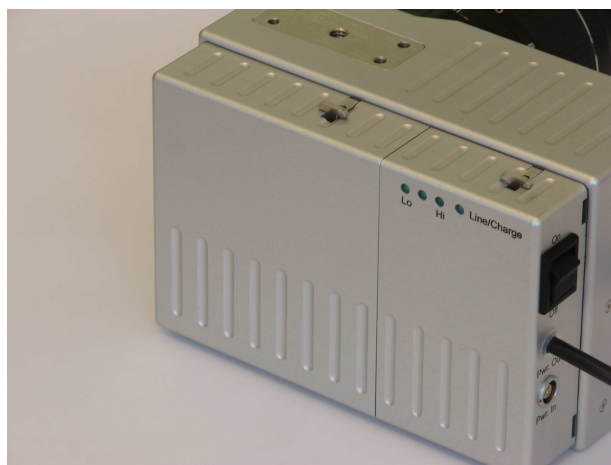
Step 5: Shift Accumulator to the right into locking position
